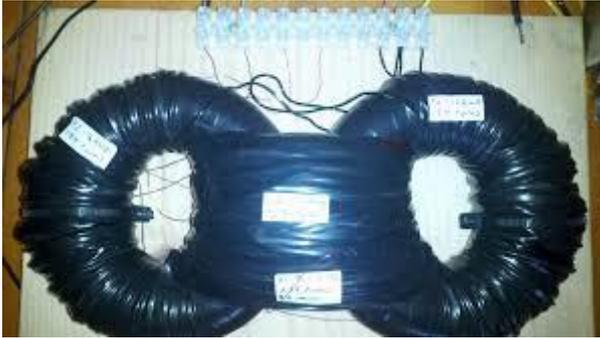
2. To energize **multiple toroids**, linking them together sequentially (the primaries in series and the secondaries in parallel), eventually putting one inside the other (the smaller ones inside).
